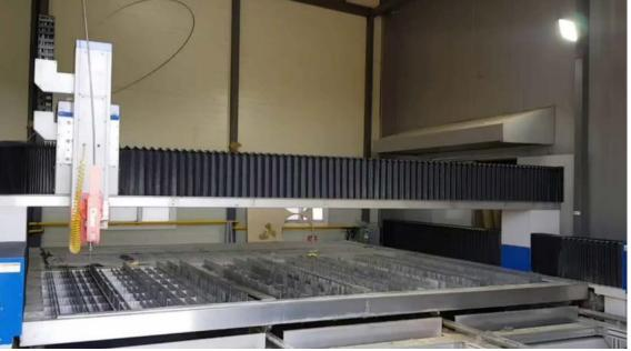
CNC waterjet cutting machine with 5 axis tilting cutting head installed
