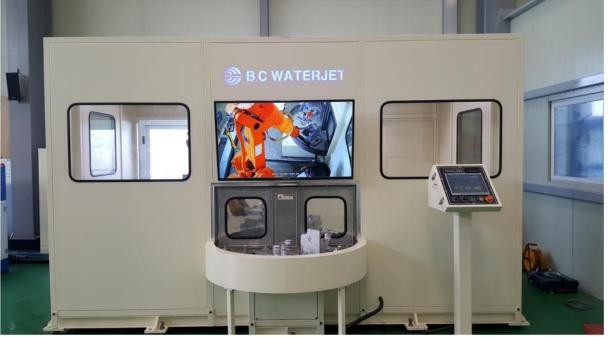
Head liner shuttle table type robot waterjet cutting with ABB IRB 2600 4 robots
