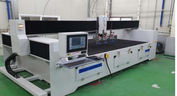
CNC waterjet cutting machine (multiple cutting nozzle installed) - Japan
