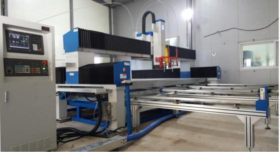
**CNC** waterjet cutting machine-Automatic loading table
