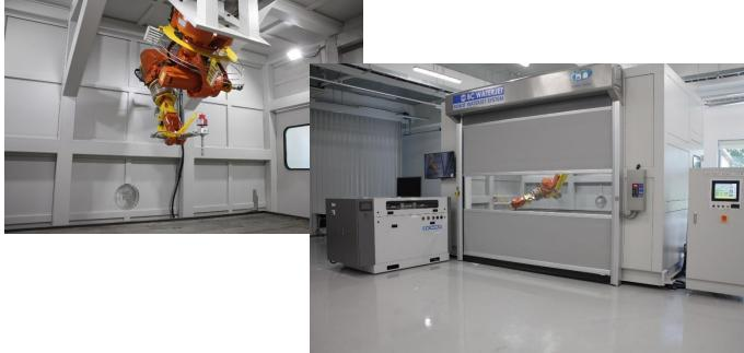
5-axis tilting cutting head waterjet cutting machine with sliding door and clean booth
